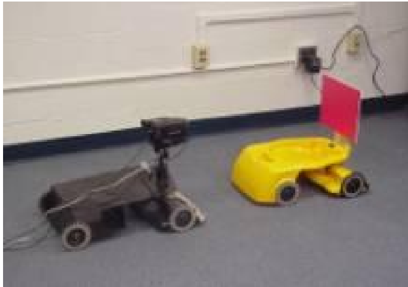
Gambar 2.1 Follower Robot Tracking Object Attached To Lead Robot
